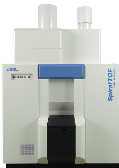
Fig.1 JMS-S3000 “SpiralTOF” with TOF-TOF attachment.
