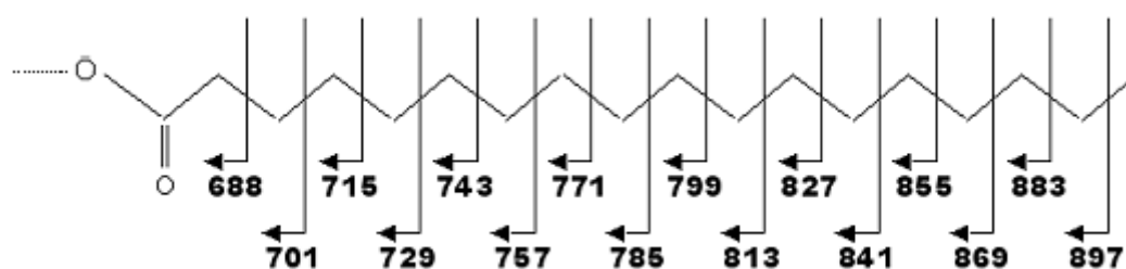
Fig.5 Peak assignment of obtained product ion spectrum.
