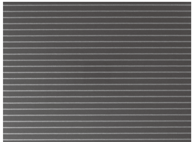
200 nm line pattern (100 kV, 100 nA).
