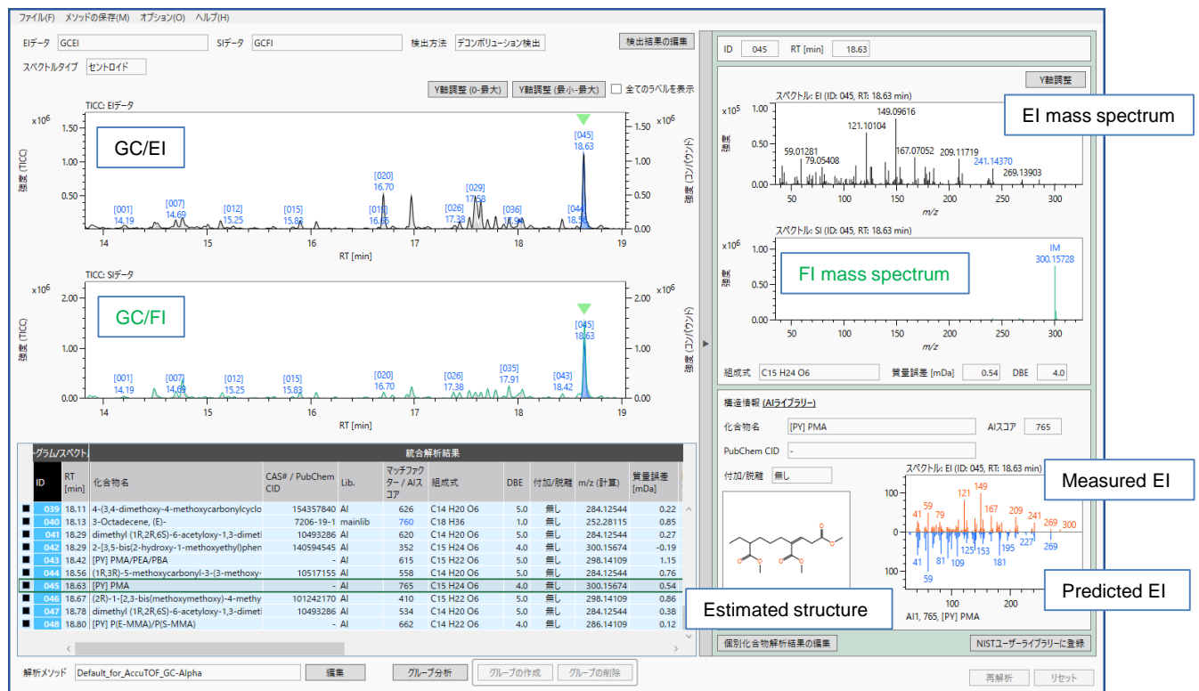
Fig.2 msFineAnalysis AI result window, ID: 045 mass spectra and estimated structure by in silico pyrolyzates
