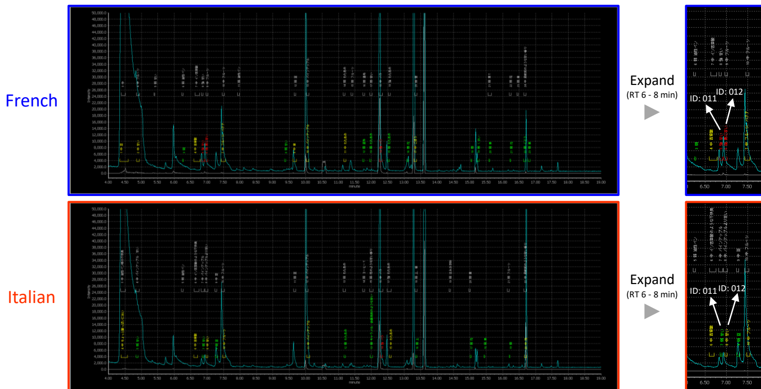
Figure 6 Integration of total ion current chromatogram (TICC) and odor information in GC-O analysis results
