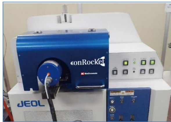
Figure 2. The ionRocket thermal desorption/pyrolysis system and DART Ion Source SVP mounted on the AccuTOF™ LC-plus 4G mass spectrometer.
