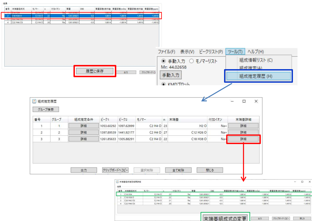
Figure 5 GUI for history of elemental composition estimations of polymers
